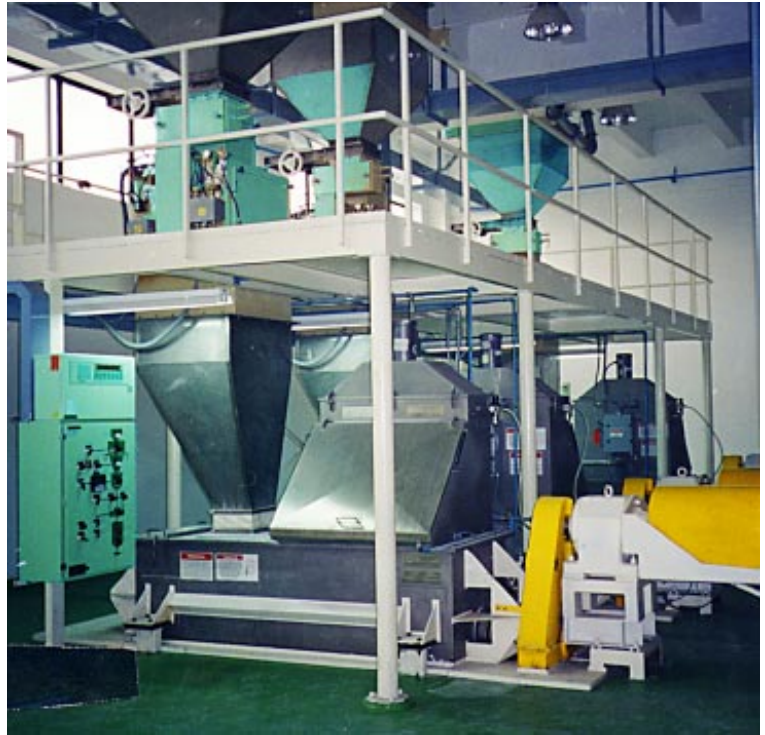
Value added sugar processor with scaling of major ingredient and filtered bag dump for minors
