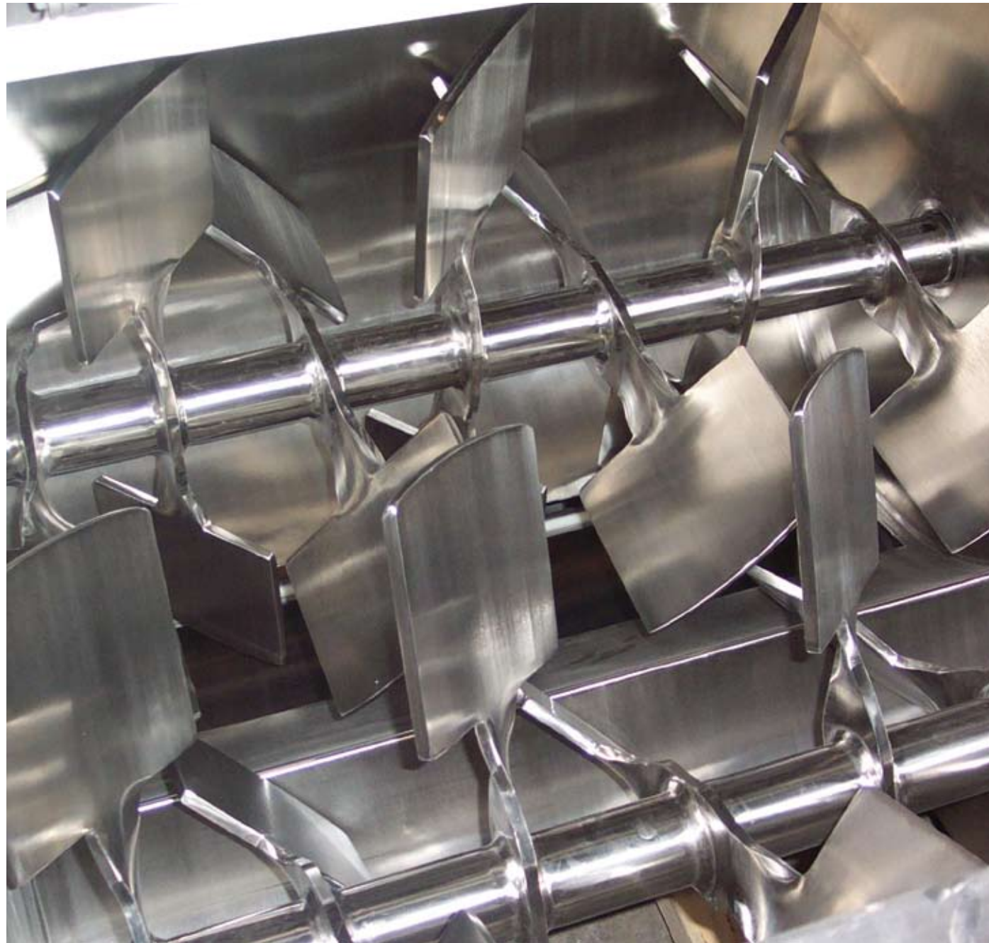
The Fluidized Zone Mixer: Overlapping and counter rotating twin shaft paddle assemblies. Shown with full length bomb bay doors.
