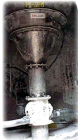
CMT reviewed numerous options with the bakery, including standard bin dischargers. In the end Carolina Conveying's Cone Valve Discharger, the Soliflo™, was chosen as the best long-term solution. This unit is bolted directly to the silo, eliminating the flexible sleeve associated with a standard bin discharger. The Soliflo™ provides two functions as well: 1) A bin activator and 2) A valve, as it completely stops product flow when closed.
