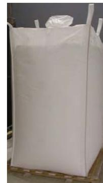
**cone table densification** of the product produces stable, safe bags without the need for internal baffles and has allowed the bag height to be reduced while still
