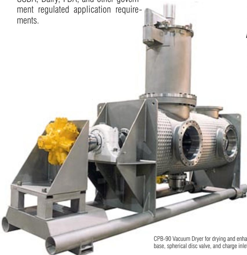
CPB-90 Vacuum Dryer for drying and enhancing the color of organic pigment. Unit has hydraulic drive, tubular load cell base, spherical disc valve, and charge inlet with davit arm.
