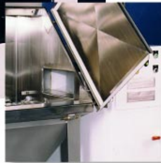
Model PBC-50 Bag Compactor (door removed to show interior; inset shows flange to bag dump)
