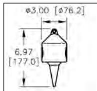
**316 Stainless Steel** – For use with corrosive solids and foodstuffs with bulk densities greater than 20lbs/ft<sup>3</sup> (320kg/m<sup>3</sup>). This plumb bob is typically shipped as a separate item, but can be assembled to the SMU at the factory upon request.
