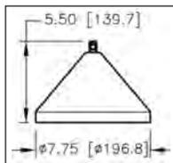
**6in. (152mm) Diameter 316 SS Ball Float** - For use with liquids with a minimum specific gravity of 0.85. A Teflon<sup>®</sup>-coated version is also available for corrosive or sticky materials. This plumb bob is shipped as a separate line item and must be attached to the cable in the field.
