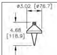
**316 SS Inverted Cone** – For use with light bulk solids and foodstuffs with bulk densities greater than 5lbs/ft<sup>3</sup> (80kg/m<sup>3</sup>). Teflon<sup>®</sup>-coated also available for corrosive or sticky materials. This is shipped as a separate line item and must be attached to the cable in the field.
